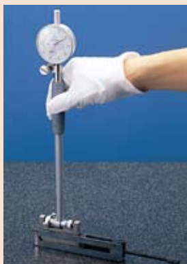
Setting a bore gage using a holder with the pair of Type I half-round jaws arranged as flat contact surfaces
