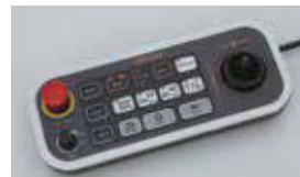
Remote box with user-friendly operability
