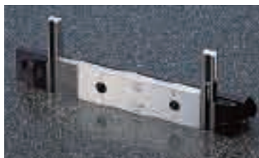
Use of B-type connectors in gage construction
